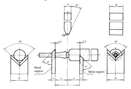
Figure Set-up for determining the breaking force of glass ampoules
